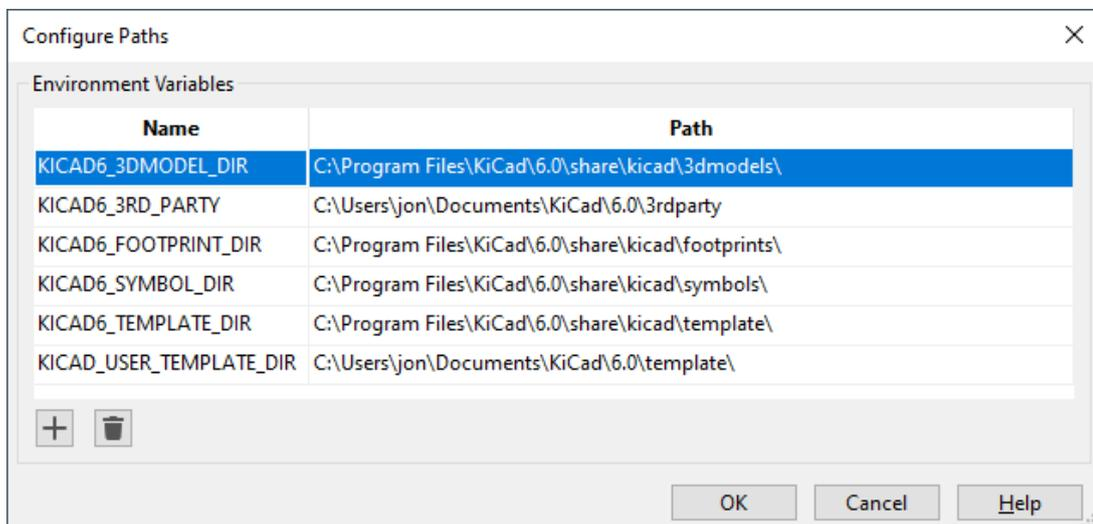
Paths set in the Configure Paths dialog are internal to KiCad and are not visible as environment variables outside of KiCad. They are stored in [KiCad's user configuration files](#).
