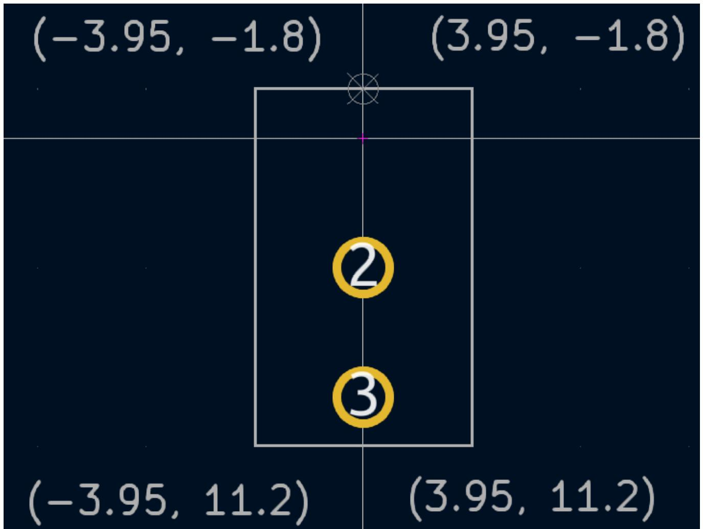
Next, switch to the **F.Silkscreen** layer. The silkscreen outline should be just outside of the part outline, so the silkscreen lines are moved outwards from the fabrication drawing by 0.11 mm. The exact coordinates are shown in the screenshot below, and helpful grid settings are:
