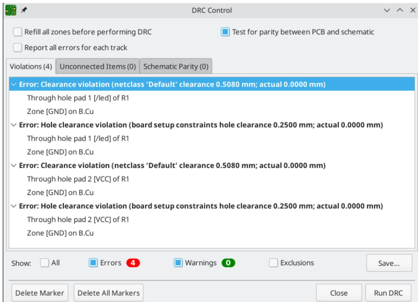
Close the DRC dialog, press kbd:[B] to refill the zone, and re-run DRC. Alternatively, check the *Refill all zones before performing DRC* checkbox and re-run DRC. All violations are fixed.
