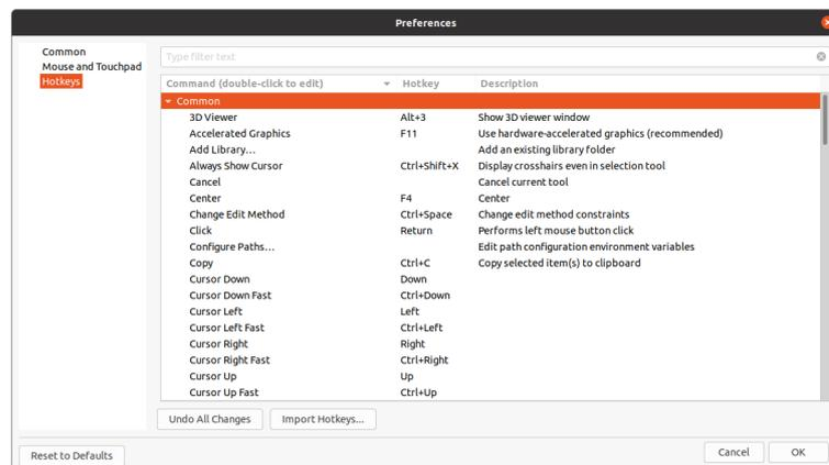
You can use this dialog to customize the hotkeys used to control KiCad. The hotkeys in the *Common* section are shared between every KiCad program. Hotkeys for each specific KiCad program are shown when that program is running. You can assign the same hotkey to a different action in different KiCad programs (for example, the schematic editor and the board editor), but you cannot assign a hotkey to more than one action in the same program.
