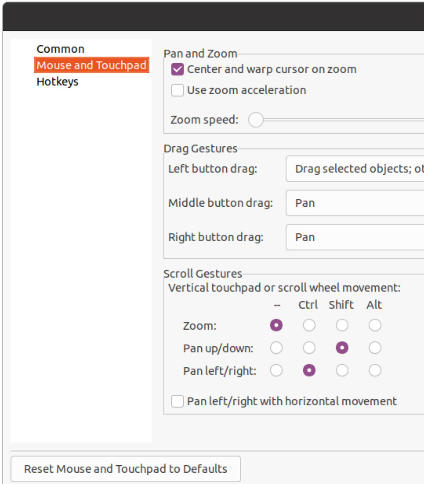
**Center and warp cursor on zoom:** When enabled, zooming using the hotkeys or mouse wheel will cause the view to be centered
