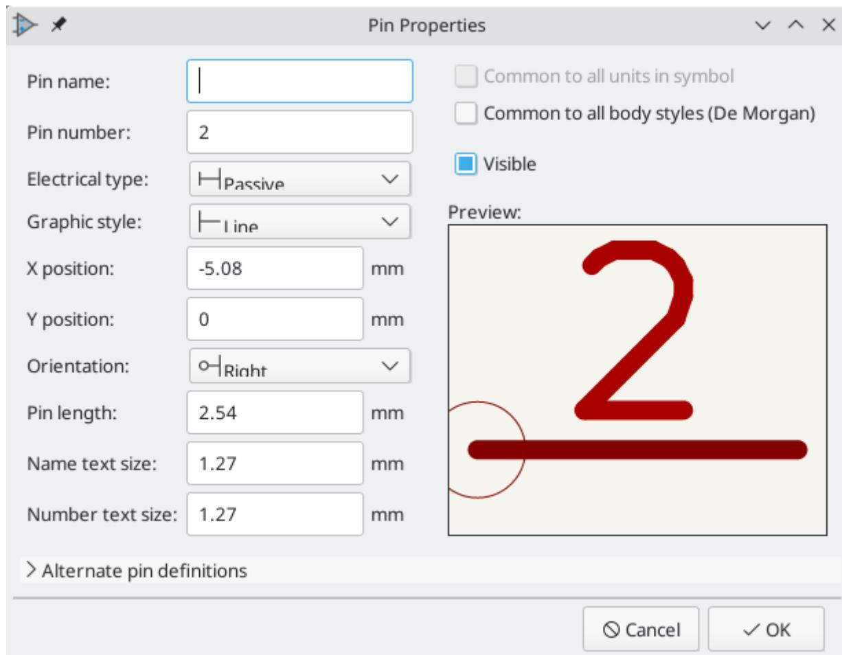
Add a second pin, but this time don't use the **Add a pin** tool. Instead, press `kbd:[Insert]`. A new pin numbered 3 is added to the symbol, just below pin 2.
