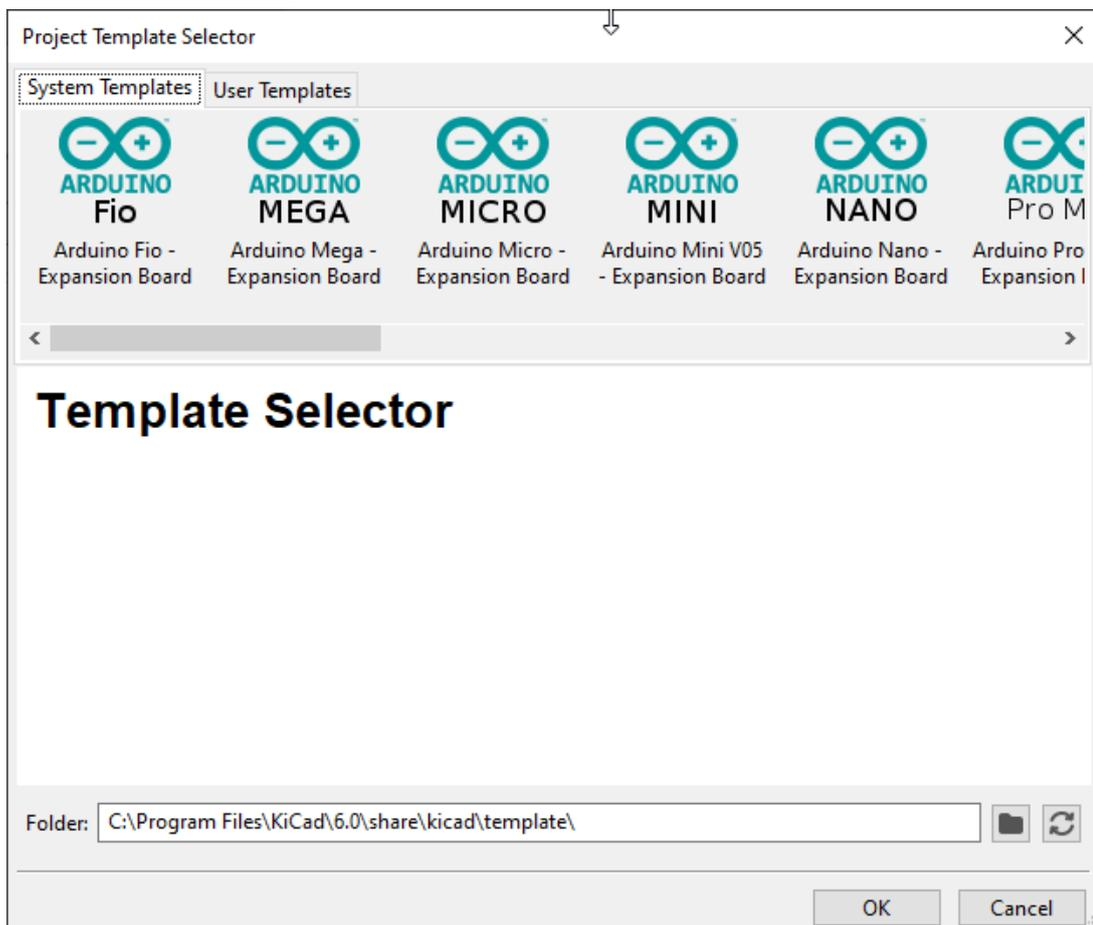
A single click on a template's icon will display the template information, and a further click on the OK button creates the new project. The template files will be copied to the new project location and renamed to reflect the new project's name.
