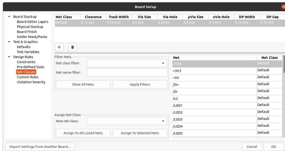
The upper portion of the Net Classes section contains a table showing the design rules that apply to each net class. Every class has values for copper clearance, track width, via sizes, and differential pair sizes. These values will be used when creating tracks and vias unless a more specific rule overrides them (see Custom Rules below).
