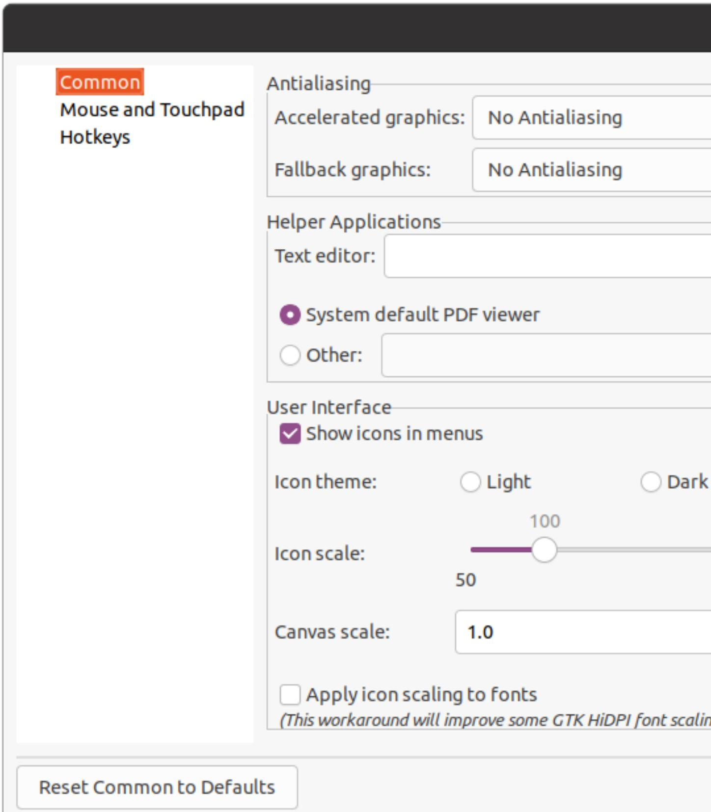
**Accelerated graphics antialiasing:** KiCad can use different methods to prevent aliasing (jagged lines) when rendering using a graphics card. Different methods may look better on different hardware, so you may want to experiment to find the one that looks best to you.
