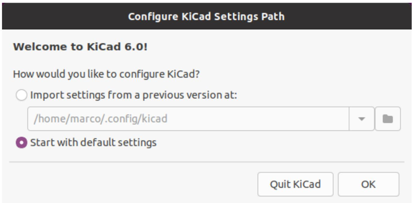
If a previous version of KiCad is detected, you will have the option to import the settings from that version. The location of the previous configuration files is detected automatically, but you may override it to choose another location if desired.
