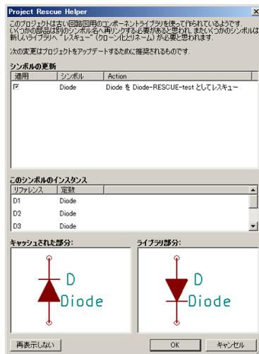
You can see in this example that the project originally used a diode with the cathode facing up, but the library now contains one with the cathode facing down. This change would break the schematic! Pressing OK here will cause the symbol cache library to be saved into a special `rescue` library and all the symbols are renamed to avoid naming conflicts.
