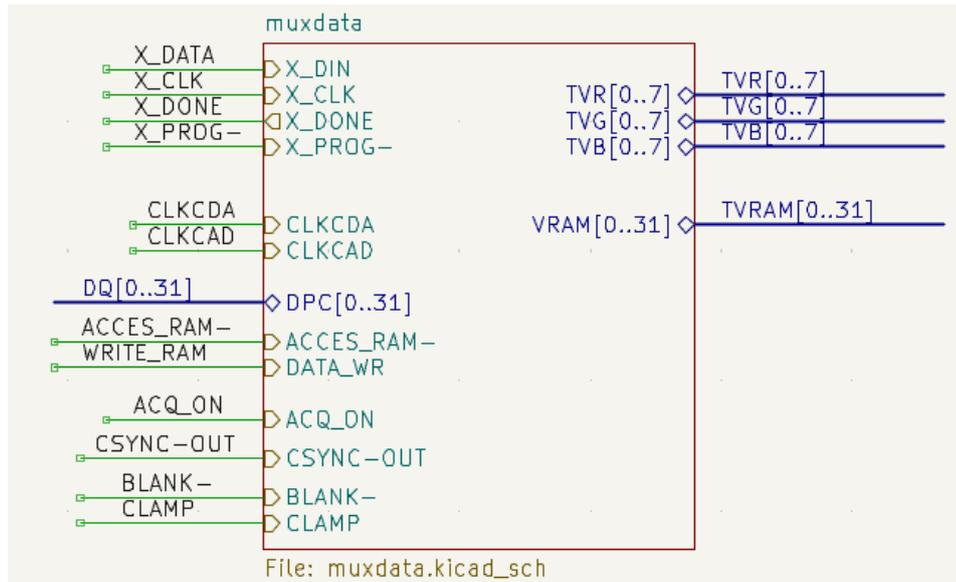
For every hierarchical label in the subsheet, import the corresponding hierarchical pin into the sheet symbol by clicking the
