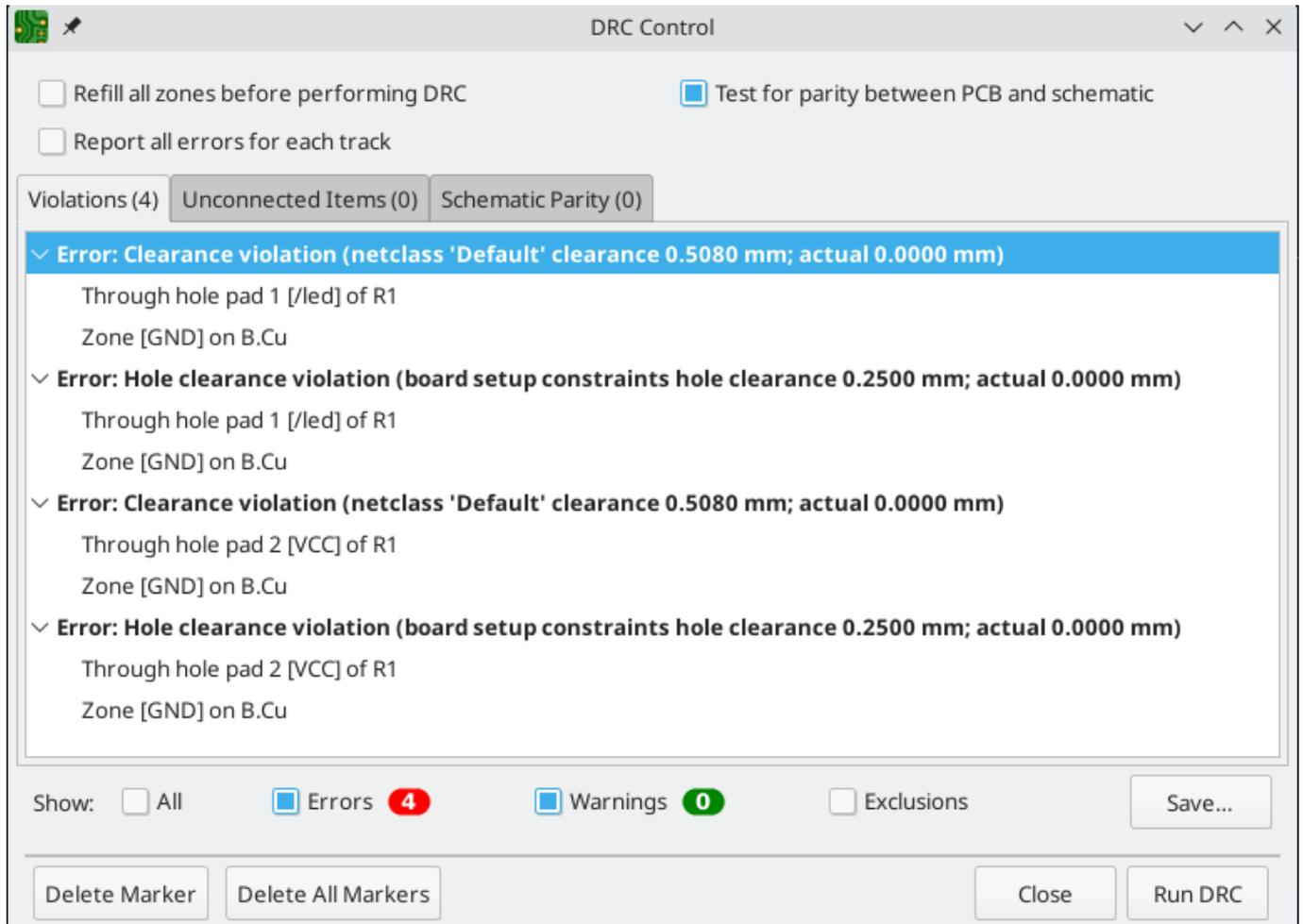
Close the DRC dialog, press `kbd:[B]` to refill the zone, and re-run DRC. Alternatively, check the *Refill all zones before performing DRC* checkbox and re-run DRC. All violations are fixed.
