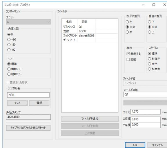
The Symbol Properties window displays all the fields of a symbol in a table. New fields can be added, and existing fields can be deleted, edited, reordered, moved, or resized.
