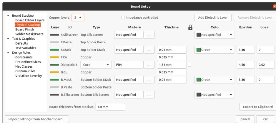
Set the number of copper layers in the upper left corner and then enter the physical parameters of the stackup if desired. These parameters may be left at their default values, but note that the board thickness value will be used when exporting a 3D model of the board. If you plan to use this feature, it is a good idea to ensure that the stackup thickness is correct.
