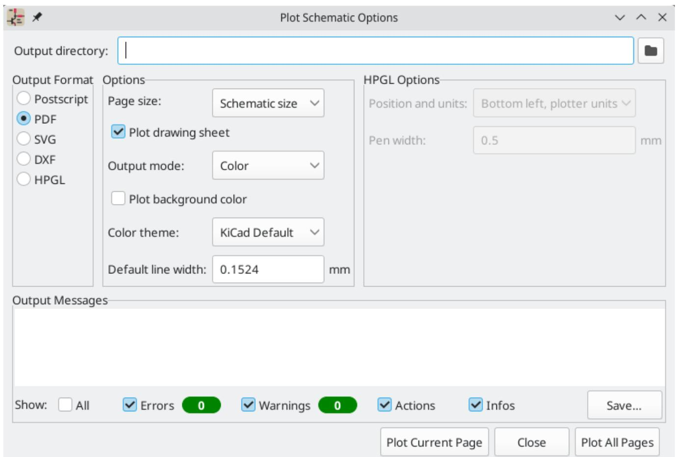
The **Output Messages** pane displays messages about the generated files. Different kinds of messages can be shown or hidden using the checkboxes, and the messages can be saved to a file using the **Save...** button.
