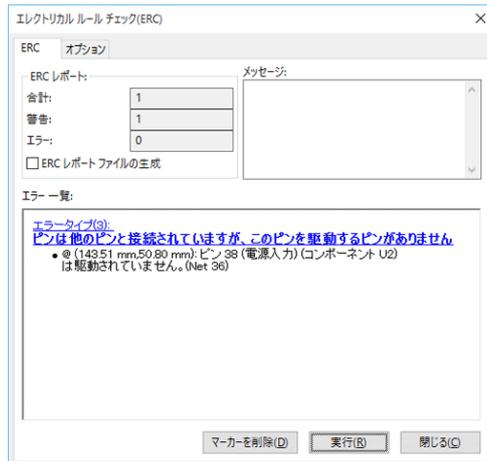
Any warnings or errors are reported in the **Violations** tab, and markers for each violation are placed in the schematic so that they point to the relevant part of the schematic. Warnings are indicated by yellow arrows, and errors have red arrows. Excluded violations are shown as green arrows.
