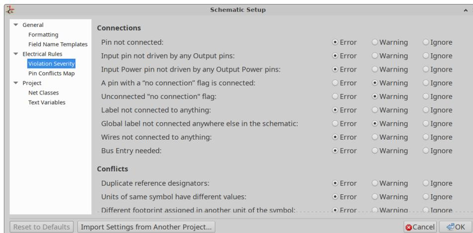
The *Violation Severity* panel in [Schematic Setup](#) lets you configure what types of ERC messages should be reported as Errors, Warnings or ignored.
