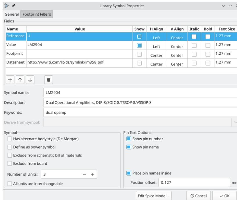
It is important to correctly set the number of units per package and the alternate symbolic representation, if enabled, because when pins are edited or created the corresponding pins for each unit will be affected. If you change the number of units per package after pin creation and editing, there will be additional work to specify the pins and graphics for the new unit. Nevertheless, it is possible to modify these properties at any time.
