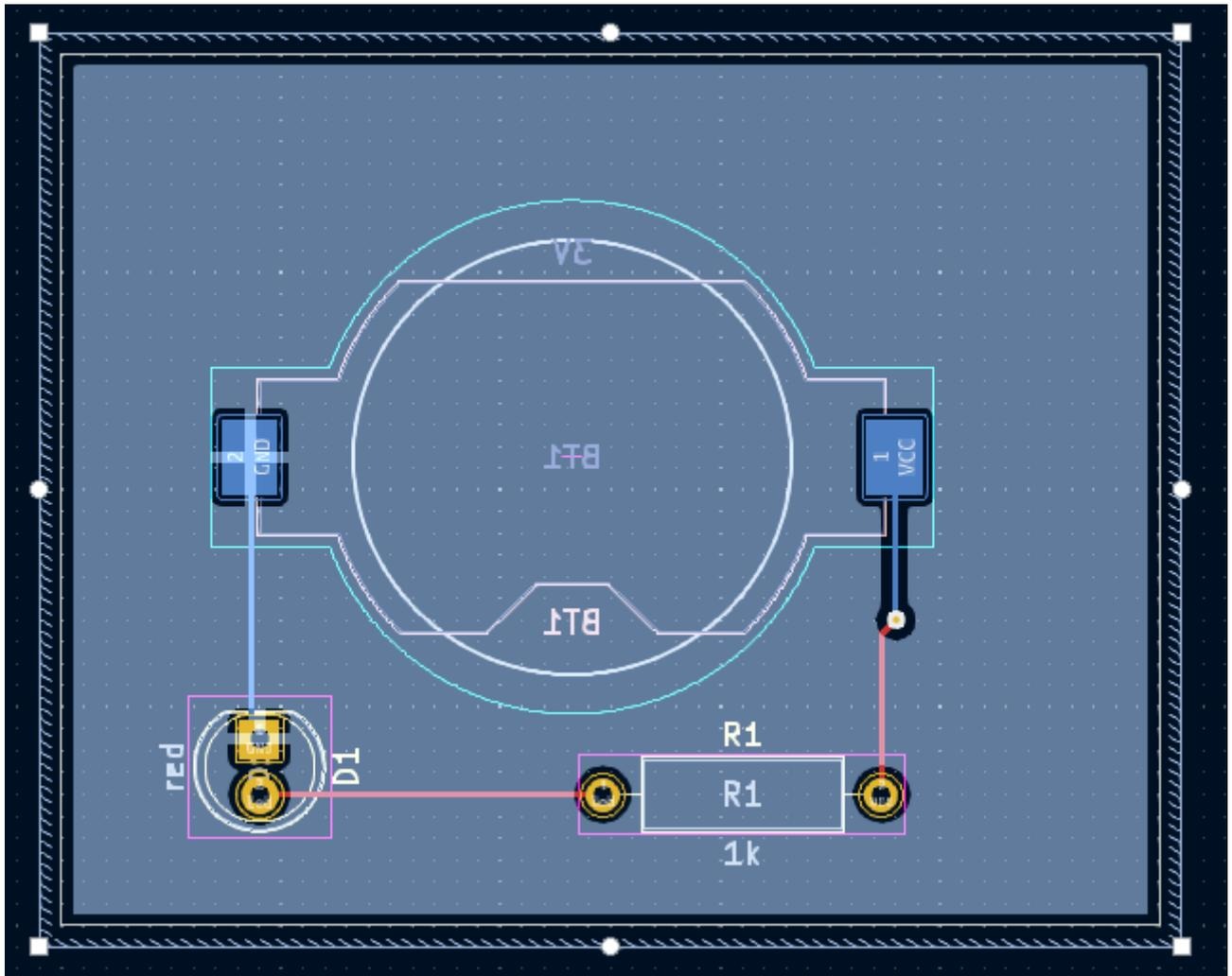
In KiCad, zones are not filled automatically when they are first drawn or modified, or when footprints within them are moved. Zones are refilled by manually filling them and when running [DRC](#). Make sure zone fills are up-to-date before generating [fabrication outputs](#).
