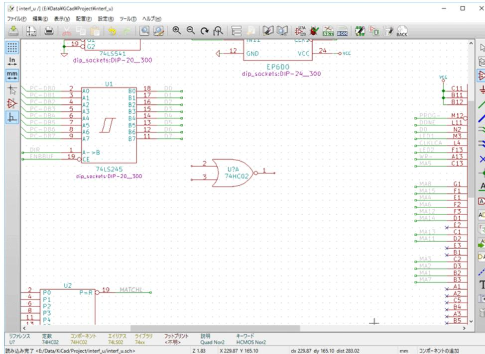
If the **Place repeated copies** option is checked, after placing a symbol KiCad will start placing another copy of the symbol. This process continues until the user presses kbd:[Esc].
