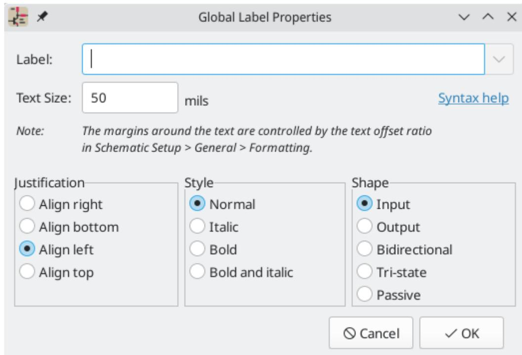
The **Label** field sets the label's text, which determines the net that the label assigns to its attached wire. Label text supports [markup](#) for overbars, subscripts, etc., as well as [variable substitution](#). Use the [Syntax help](#) link in the dialog for a summary.
