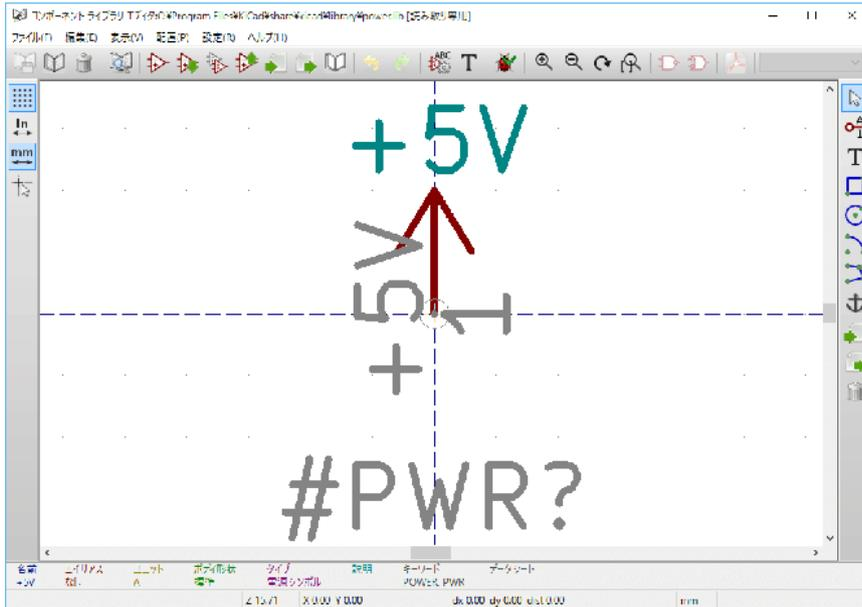
Power port symbols consist of a pin of type "Power input" that is marked invisible. They must also have the "Define as power symbol" property checked. Invisible power input pins have a special property of making implicit global connections based on the pin name.
