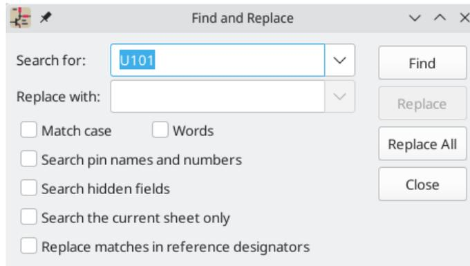
If the **Replace matches in reference designators** option is checked, reference designators will be modified if they contain matching text. Otherwise reference designators will not be affected.
