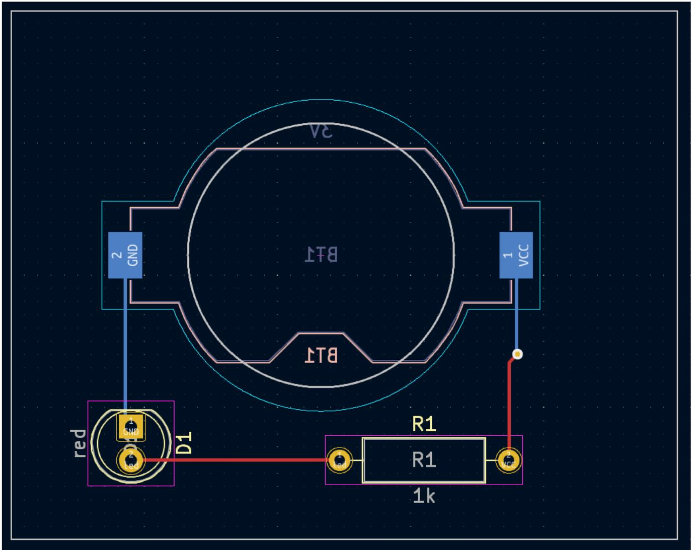
At this point, all connections are routed. This can be confirmed by looking at the status screen in the bottom left of the window, where the number of unrouted nets is given as 0.
