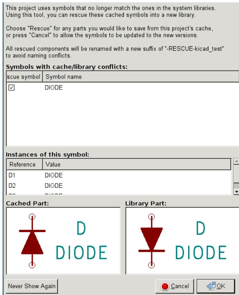
You can see in this example that the project originally used a diode with the cathode facing up, but the library now contains one with the cathode facing down. This change would break the schematic! Pressing OK here will cause the symbol cache library to be saved into a special `rescue` library and all the symbols are renamed to avoid naming conflicts.
