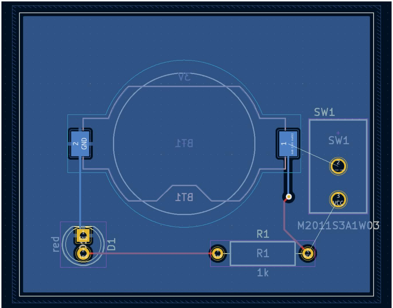
The ratsnest shows the new connections that need to be routed. Additionally, the connection between the battery and the resistor needs to be deleted.
