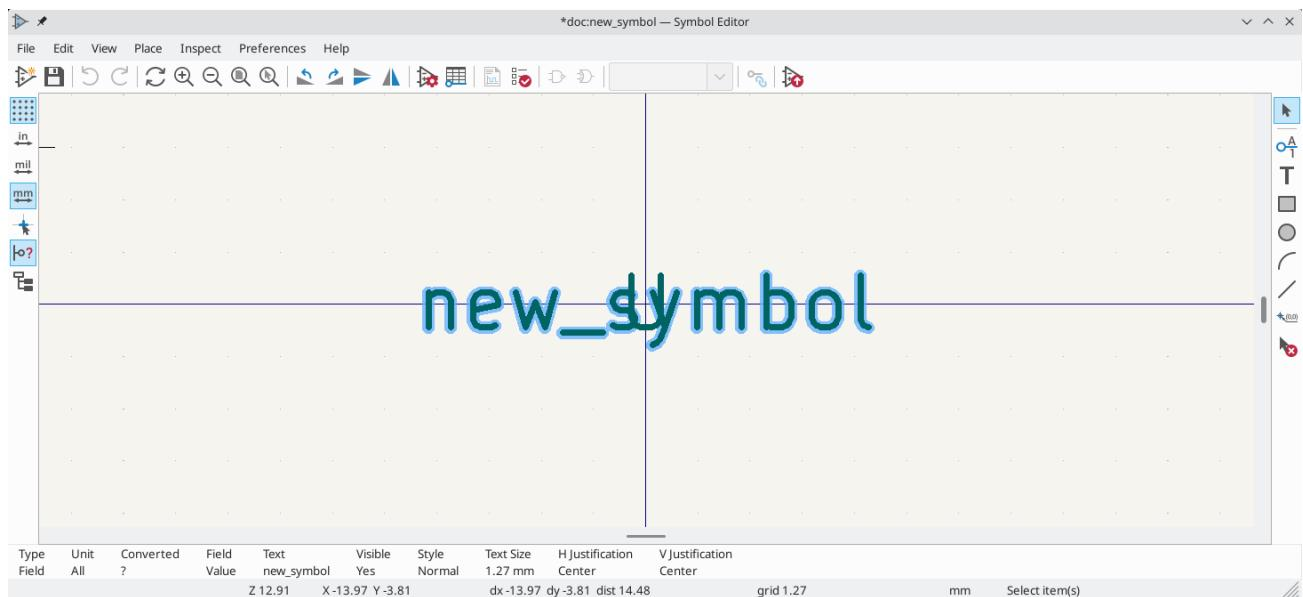
The blue cross in the center is the symbol anchor, which specifies the symbol origin i.e. the coordinates (0, 0). The anchor can
